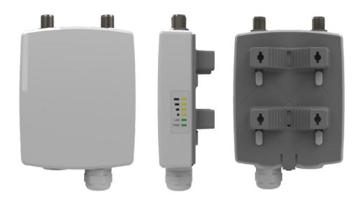
The WIP5800N-WR is a versatile, very efficient, and stable 5 GHz wireless access point. The unit is equipped with an extreme output power (up to 29 dBm) 802.11n MIMO radio wrapped securely inside a robust IP-65 compliant enclosure with two N-type connectors, suited for wide coverage area applications.
