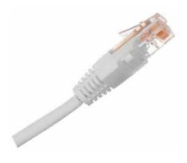
This 1 ft. gray category 5e (Cat5e) patch cable has 2 standard RJ45 molded male connectors featuring integral strain relief. The cable is manufactured from PVC 4-pair stranded UTP and is rated for 350 MHz/1 Gbps communication. Cabling for category 5 (Cat5) and 5e (Cat5e) applications. Meets most current industry standards including IEEE 802.3ab, IEEE 802.5, ANSI/EIA/TIA 568, ISO/IEC 11801 and ETL.
